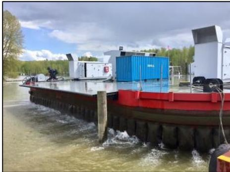
450 tonne payload capacity is now ready-to-work. For over fifty years, specialized hover barges have proven to be cost-effective solutions for transport of heavy loads over environmentally challenging
