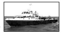
**File: CB10047 Crew Boat:** 100.1' loa x 21.0' beam x 10.7' depth x 4.76' loaded draft. Built in 2005 by Grandweld Shipyards; UAE. Kuwait flag. GRT: 127. Class: BV I, Crewboat Service Restriction: Arabian Gulf. Light Disp.: 80T. Deck Cargo: 25T on 65m2 clear deck. Main Engines: 2 x Cummins KTA38-M2 total 2,800BHP. **Speed about 18.5kn**. Genset(s): CAT. **Passengers: 24**. Owner is open to scrap offers. Call Marcon for guidance. **Mid East.**
