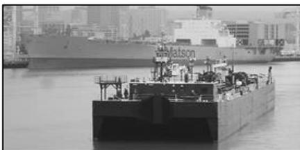
A U.S. flag, single-hull, 45,000bbl tank barge was sold on a private & confidential basis. The barge measures 300.0’ x 56.0’ x 21.5’ depth and was built in 1971 by Gretna Machine & Iron Works of Harvey, Louisiana for petroleum service on behalf of one of the oil majors. Barge was classed ABS +A1 Oil Tank Barge. The 6,153dwt barge is being converted to alternate service. Marcon was the sole broker.
